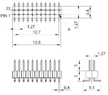
Figure 3: Typical pin header for vehicles
