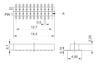
**Figure 2:** Typical socket connections for decoders
