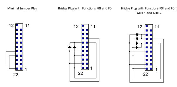
Figure 6: Typical Jumper Plugs
