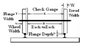
Back-to-Back, B, is derived by knowing B = K-T. K is the primary controlling dimension.
