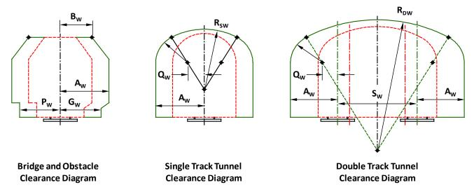
Following guidance from the **AREA** and **AREMA**, the figure above shows the required modifications using green lines. For visual reference, the red dashed lines represent the tangent track clearance diagrams from the figures in **NMRA RP-7.1**. Any dimensions the figure above *does not* show remain the same as those tabulated in **NMRA RP-7.1**. The addition of the subscript **W** (for "wider") means a new value you must calculate using the simple instructions below.
