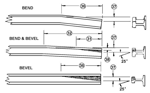
The Flare leading into the flangeway formed by Guard and Wing Rails may be made by bending the end of the rail, by machining a Bevel, or by a combination of both Bend and Bevel.
