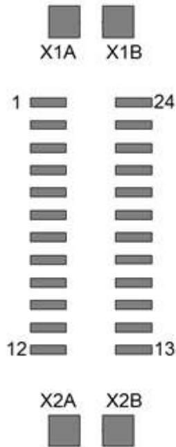
Figure 7: Pin Arrangement for E24 Interface
