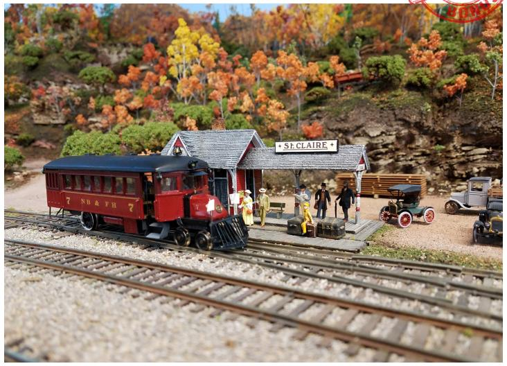
▲ Here's a snap taken of the NB&FH railbus as it is stopped at the St. Clair station. It started life as a Jordan Highway miniatures kit. A new brass frame, wheels, can motor, and sound decoder, were added. She now alerts passengers using an aa-uu-gaa! and a bell.
