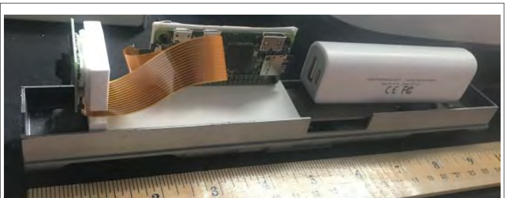
A Raspberry Pi Zero W, camera, and power bank loaded onto an old Tyco passenger car chassis will serve as a wireless train cam for upcoming remote ops sessions. The car will receive a special 3D printed locomotive body which will blend in with the powered locomotives. The car will run on the head end of assigned trains and the image will be viewable on a web browser.
