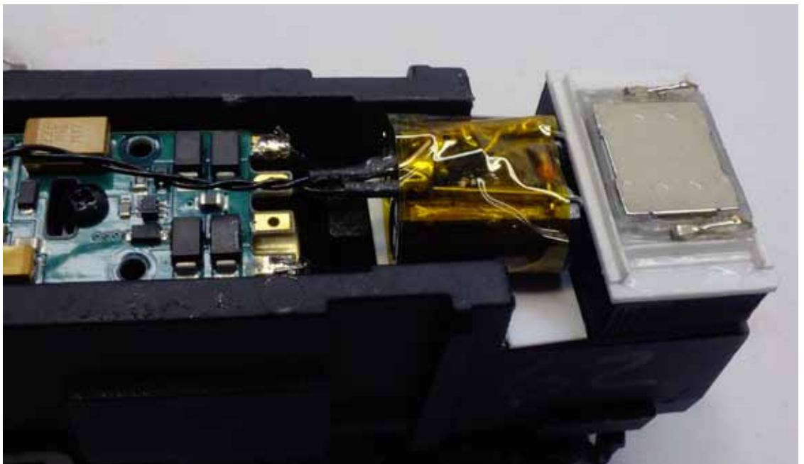
Figures 11 and 12: KA made with two 1000uF Capacitors in series for Stewart F7A, located in rear of chassis.
