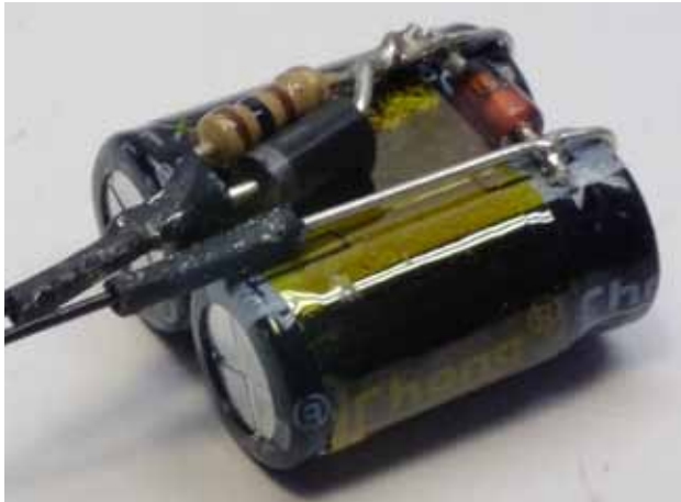
Figures 11 and 12: KA made with two 1000uF Capacitors in series for Stewart F7A, located in rear of chassis.
