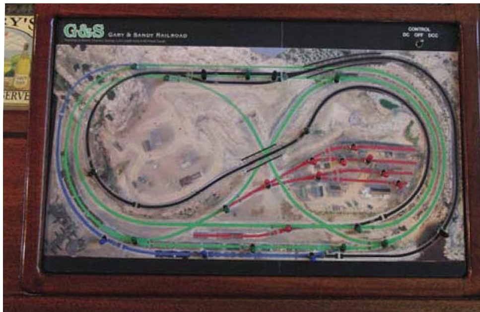
G&S Railroad control panel can be operated in either DC or DCC modes
