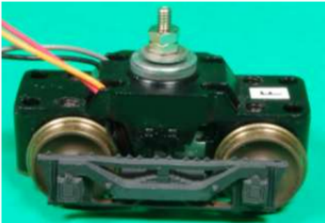
▲The NWSL Stanton drive with AMB side frames. Note the “F” to denote which end faces the front of the locomotive.
