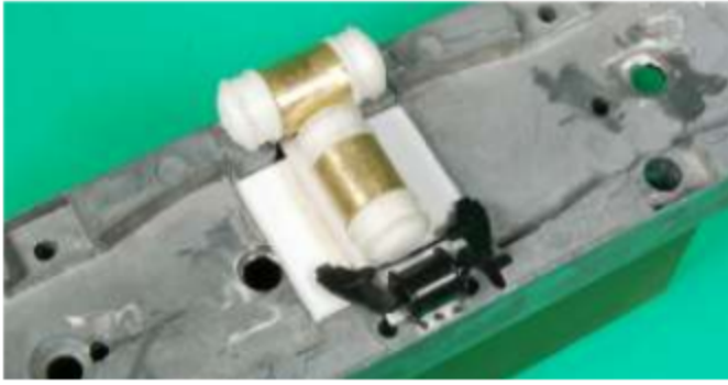
▲The air tanks and brake cylinder, after installation.
