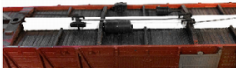
The one-piece brake rigging is cemented to the Evergreen straight frame sills. This is the extent of the underbody detail.
