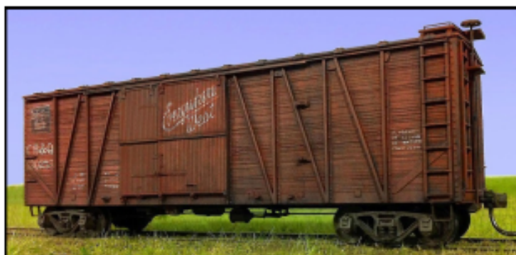
Above is my most recent Accurail model. I added the extra door to make a so-called door-and-a-half boxcar. I also replaced the fish-belly frame with a straight sill frame, and then added Accurail's one-piece brake rigging. Otherwise the model is a factory painted Accurail CB&Q kit.
