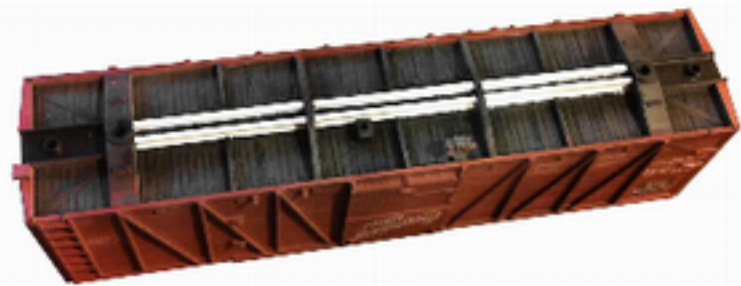
This is an Accurail outside-braced wooden boxcar. The fish belly frame was discarded to the scrap box and a straight frame installed using Evergreen 1/8" C-channel installed back-to-back into the slots for the fish-belly frame...
