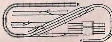
fiddle level with through station and multiple sidings ramp made of Märklin bridges to upper level layout size: 350 x 130 cm (11' 5" x 4' 4")
