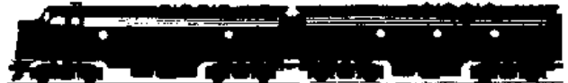
2(B-B) GM FP7 1500 HP "A" and "B" Units Frt. and Pass. Service
