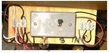
You may use 18 or 16 gauge stranded wire for the connections to the lamp and switch, as you prefer. I strongly recommend that you get the iron really hot. I used a 25 watt ordinary Weller. Once the iron is hot and solder flows easily, clean the side of the lamp base with emery paper or a file. Flux and solder quickly. Once done, do the contact on the bottom, once and really fast. Do not keep the iron there, the lamp will come apart.
