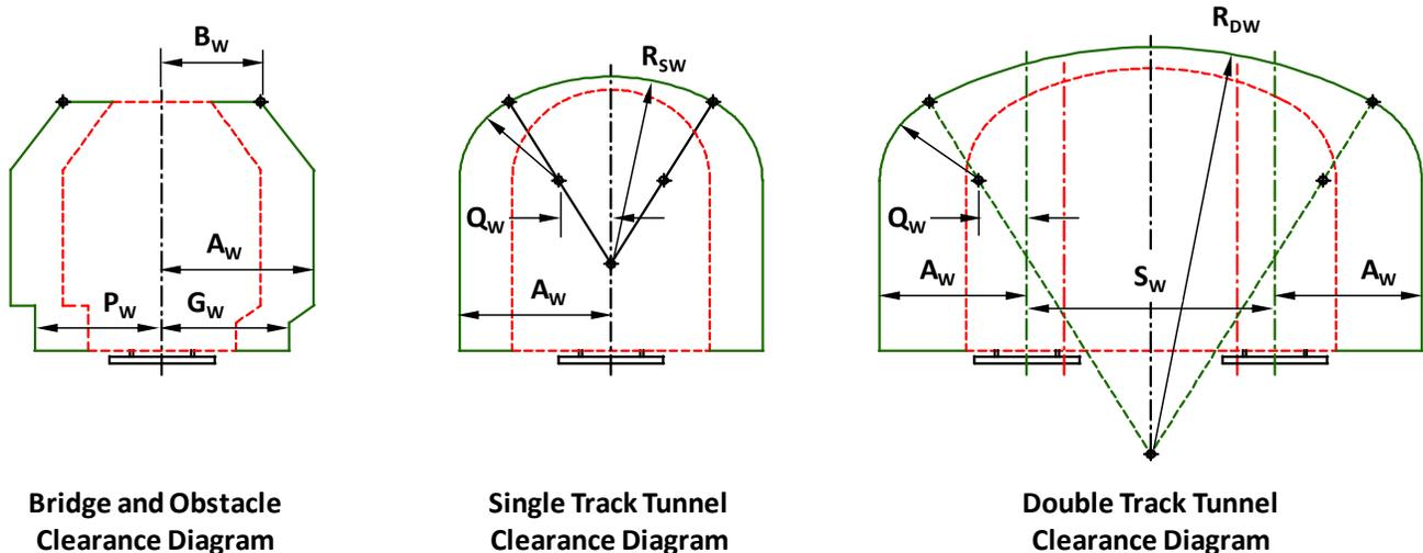
Following guidance from the **AREA** and **AREMA**, the figure above shows the required modifications using green lines. For visual reference, the red dashed lines represent the tangent track clearance diagrams from the figures in **NMRA RP-7.1**. Any dimensions the figure above *does not* show remain the same as those tabulated in **NMRA RP-7.1**. The addition of the subscript **W** (for “wider”) means a new value you must calculate using the simple instructions below.
