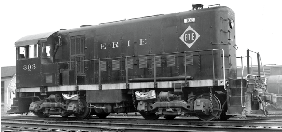
Below: The Erie bought four HH660s very near the end of production. We show the 303 working in Jersey City on April 2, 1957, with two rerrail frogs on hangers above each truck on this side, as well as a pushpole bracketed on the running board: Erie is ready for anything. This is a final phase HH660, not differing in any substantial way from all production after the 1938 revision of the carbody.
